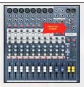
If the mic uses a voltage from the mixing board that voltage has been standardized at 48 volts. We call this voltage phantom power. Most consoles large and small will have a button to engage phantom power clearly marked. The backplate of the condenser mic retains a negative charge, the front plate or diaphragm, maintains a positive charge and an
